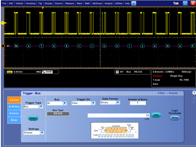
Capture – Triggering on a specific transmit data packet going across an RS-232 bus. A complete set of triggers, including triggers for specific serial packet content, ensures you quickly capture your event of interest.
