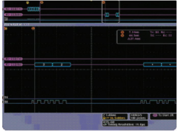
Figure 25. RS-232 triggering and decoding on the DPO4000.
