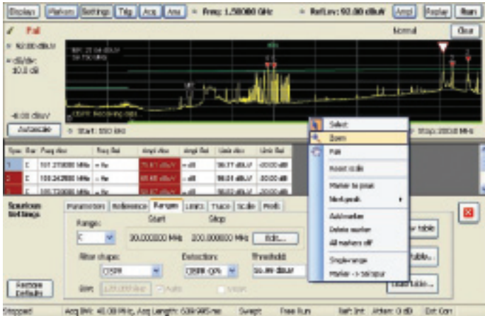
Figure 2. A scan of ambient signals from 150 kHz to 200 MHz. Quasi-Peak detection is used for the entire scan. The spurious measurement in the RSA6100A is set up to change limits vs. frequency, and antenna correction factors have been applied, resulting in the sloped noise floor of the displayed signal. Violations above the user-set limits are shown in red on the table. The menu on-screen can be used to zoom on any portion of the display for closer evaluation.
