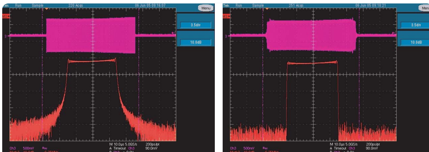
► Figure 12. Unknown targets hidden in noise (left). Compressing the power that was previously spread across a wider bandwidth so the signals (target returns) come out of the noise floor (right).
