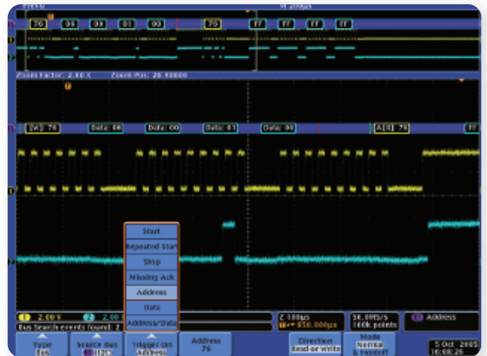
► Figure 8. The DPO4000 I 2 C Bus triggers on selected address 76 for a read or a write. Each packet is easily decoded eliminating hand decoding, reducing errors and saving time.
