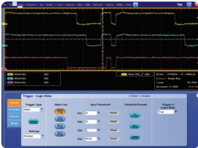
► Figure 9. A DPO display shows time qualified pattern triggering for a device. The input line for Ch 3 should be high when the signals on Ch 1 and Ch 2 go high. Setting Ch 3 to a low state uncovers an added delay problem.
