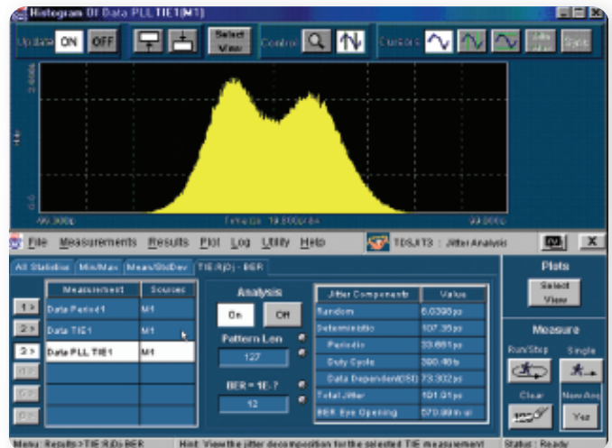
► Figure 17. DPO7000 with the TDSJIT3 Jitter Analysis application reveals a total jitter on the data signal equal to \sim 192 ps ( T_j = D_j + 2Q(\text{BER}) * R_j ), where Q(10E-12) = 7 . The associated histogram of data PLL TIE measurement provides an engineer with a graphic representation of the data signals statistical distribution.
