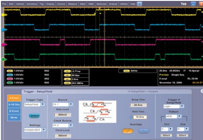
Figure 6. Logic Qualified Setup-and-Hold Triggering.
