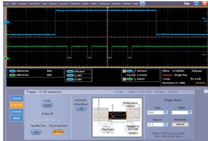
Figure 9. Triggering on Drive Defect.
