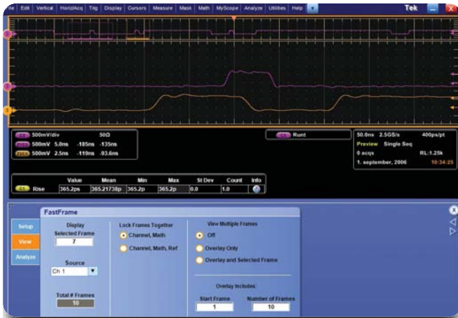
► Figure 14. A comparison of intermittent anomalies using zoom with FastFrame acquisition. Notice the Multi-zoom display used in conjunction with the selected frame to compare runt pulses on Channel 3.
