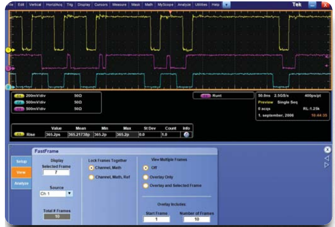
► Figure 13. Compare the conditions of each acquisition independently by scrolling through them using the VIEW menu of FastFrame.
