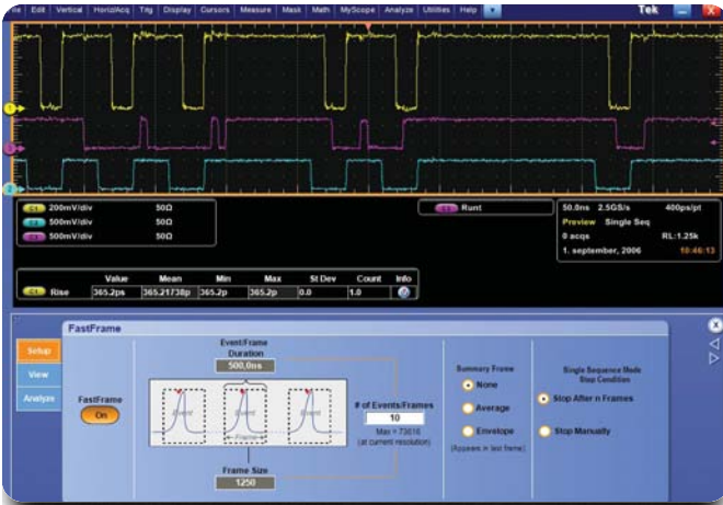
► Figure 12. A cause/effect analysis using FastFrame in multi-channel mode. Channel 1 is a data signal, channel 2 is the clock, and channel 3 is the resulting signal with runt pulses caused by a setup/hold time violation.
