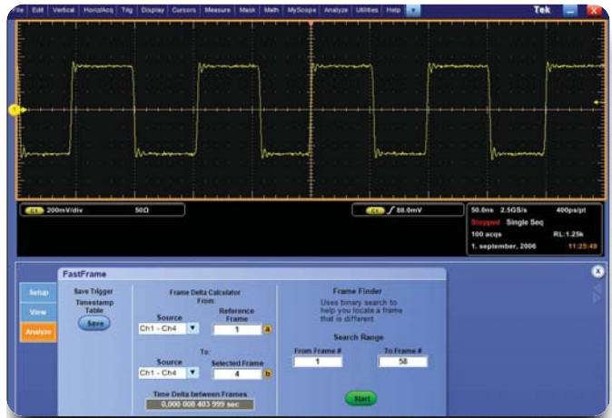
► Figure 11. FastFrame Time Stamp Snapshot display shows the relative time between microprocessor interrupts.
