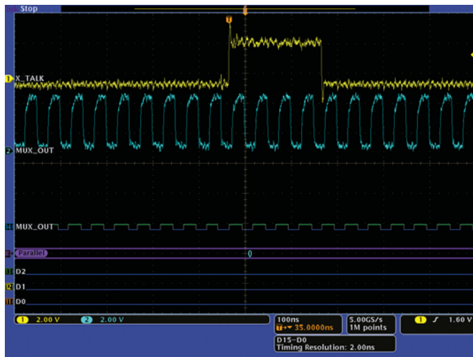
Figure 9. The PCB modification removes the crosstalk.
