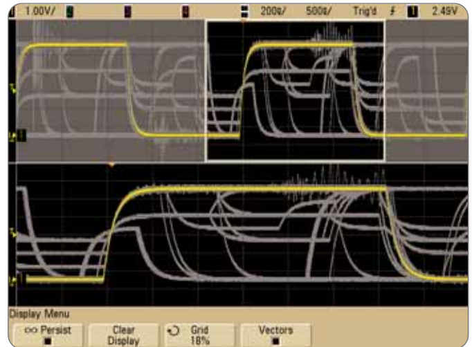
► Figure 3a. Competitive alternative approach to DPO, however the trace is monochrome and has no frequency dimension.
