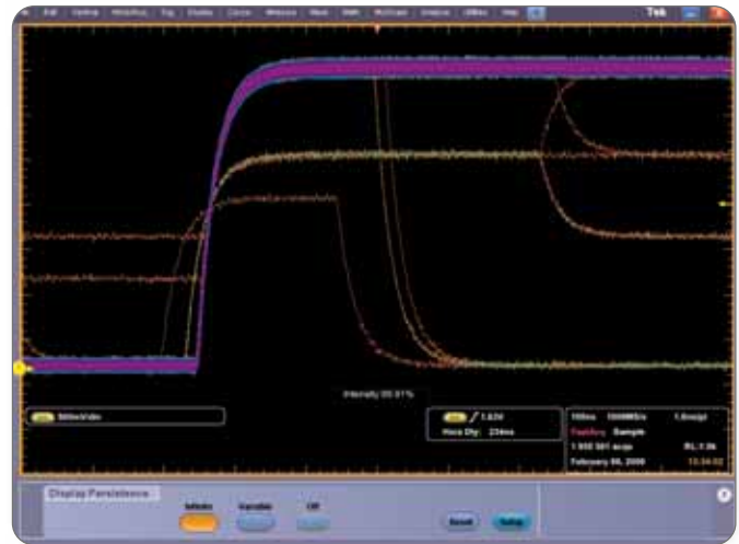
► Figure 5. The DPO highlights the aberrant traces in red. Because Persistence is set to infinite, the display maintains the trace for easy viewing and assessment.
