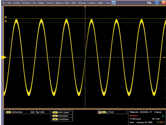
Figure 7. Side-by-Side Comparison of 6.5 GHz Sinewave on Tektronix and Agilent Oscilloscopes.
