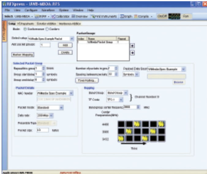
Figure 7. UWB-WiMedia signal generation in RFXpress conformance mode.
