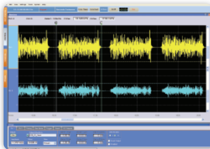
► Figure 22. UWB signals can be directly generated on the AWG7000.
