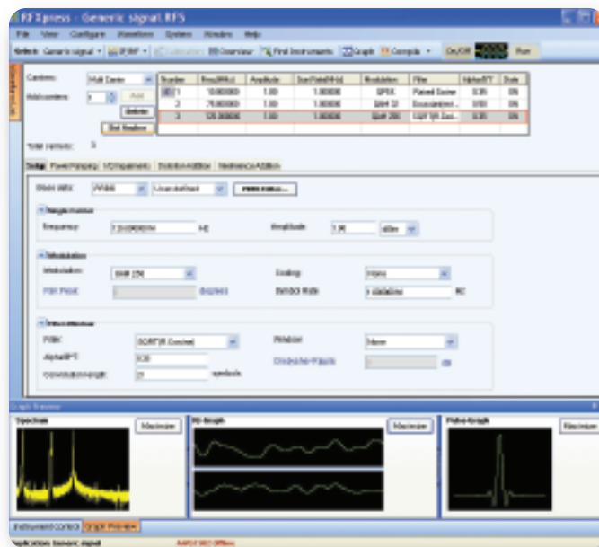
► Figure 25. RFExpress offers powerful waveform generation capabilities for Tektronix AWGs, like this multi-carrier QPSK example.
