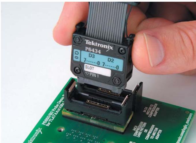
Figure 5. High-density, multi-channel logic analyzer probe.
